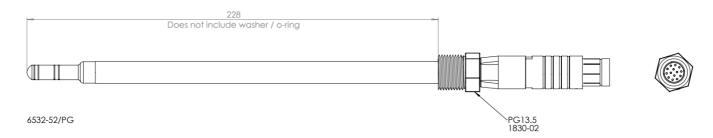
Note that this is a standard 220mm sensor with PG13.5 nut.
