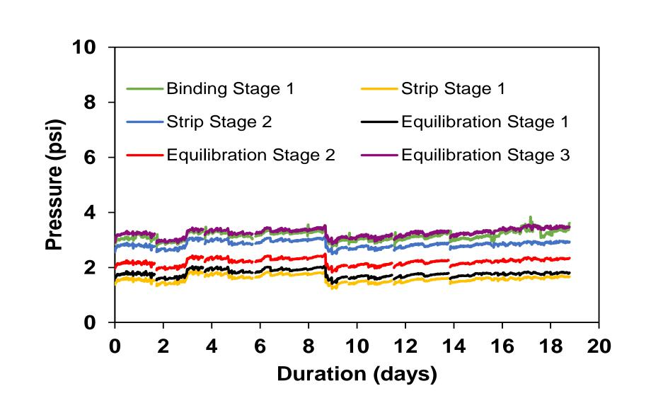
Long term stability of the CCTC system: Ideal for integration with perfusion bioreactor.
